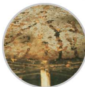
▲ Welded type air area of the STS tank : Corrosion occurs due to chloride gas.
