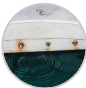
▲ When general STS bolts are used in the air area : Corrosion occurs due to chloride gas.
